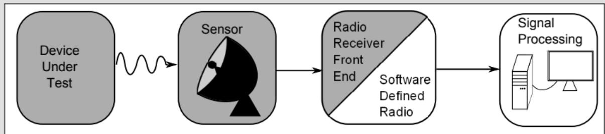
Capture the electromagnetic emanations of a device with state of the art radio equipment to use them for a side channel attack.
