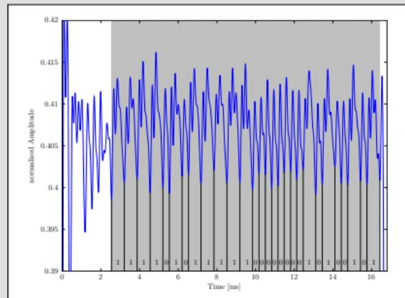
Automated averaging of multiple signal blocks makes it possible to extract key of S&M algorithm.
